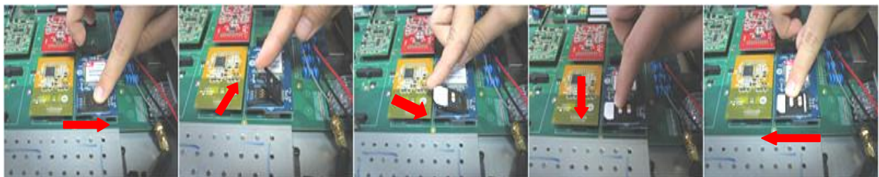
Figure 3-4 Inserting the SIM Card
